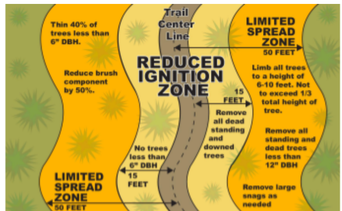
Reduced Ignition Zone diagram designed for SBTS by Ryan McCarthy, Abandoned Mine Lands Division Manager - Environmental Protection Services
